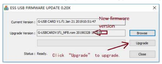
5. X26 USB MODEL will restart automatically during the upgrade process. After the green progress bar is finished, the upgrade process is complete.
