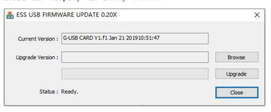
As shown in the figure below, the firmware upgrade program has displayed the current firmware version number of the X26 USB MODEL, indicating that the X26 USB has been successfully connected and the status is normal.
